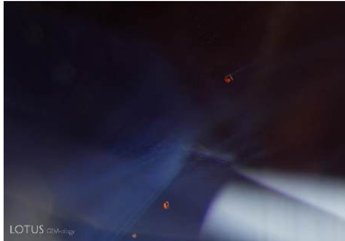
Figure 4: a tiny red octahedral of uranium pyrochlore in a Cambodian sapphire. Photographer: E. Billie Hughes. Taken on internet from Lotus gemology hyperion database ( www.lotusgemology.com/index.php/library/inclusion-gallery?filter%5Bgemtype%5D=Natural+Sapphire&filter%5Borigin%5D=Cambodia&filter%5Benhancement%5D=&filter%5Bsearch%5D=&start=0&layout=gallery#lg=1&slide=2 ). Also in Hughes, 2017
