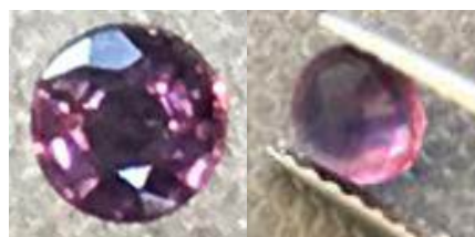
Figure 14: sample SW2 seen face up (left) displaying a purple colour, the same sample seen from bottom side showing colour zoning (pink / blue)
