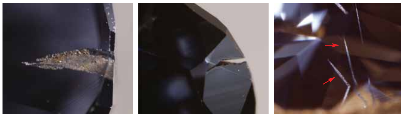
Figure 5. HGBV diamonds exhibited different types of characteristic internal features. These included (left, magnified 52×) coarsely textured channels, where chemical etching occurred along preexisting cracks or cleavages; they can sometimes be very deep, as seen in the 0.73 ct stone in the center (magnified 40×). Another type of feature (right, magnified 52×), either etch or growth tubes, consists of hollow, icicle-like acicular inclusions. Photomicrographs by C. P. Smith.
