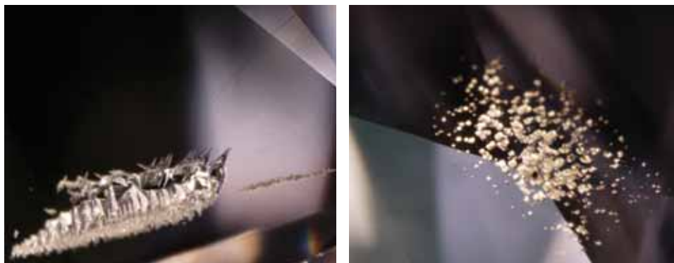
Figure 6. Also present in the HGBV diamonds were shallow cavities that resembled furrows with radiating acicular margins (left) and fields of small pits (right), which may be either etch features or remnants of inclusions removed during cutting. Photomicrographs by C. H. van der Bogert; magnified 40 \times .
