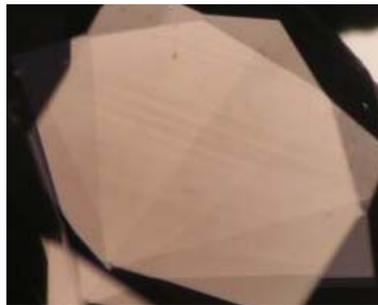
Figure 9. Graining in one {111} direction which appears to overlay near homogeneous color
