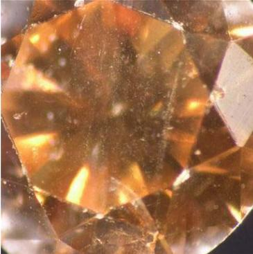
A close-up image of the diamond showing internal features, including a large, irregular, brownish inclusion. |
