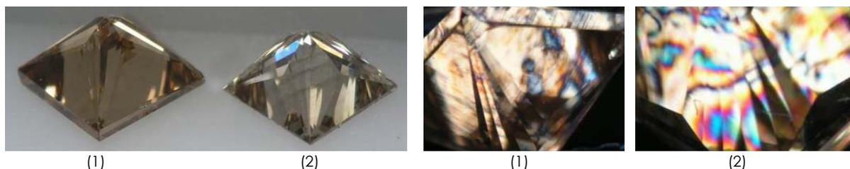
Figure 55. The strain pattern of the light brown diamond (2) is apparently much stronger than the more linear pattern of the medium dark brown diamond (1)
