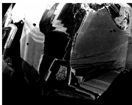
Figure 46. Irregular and step-like CL in a CO<sub>2</sub> diamond (sample 52)
