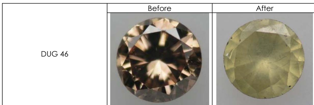
Figure 66. Sample 46 before (left) and after the HPHT treatment at 2000°C and 6.5 GPa (right, not repolished)
