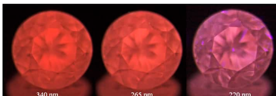
Figure 30. A pink brown type IIa diamond (sample TH 2.584) under three different UV excitations of the DFI system. The pink to orange red PL is caused by the possibly oxygen- or nickel-related 559.7, 584.5, and 597.9 nm defects.
