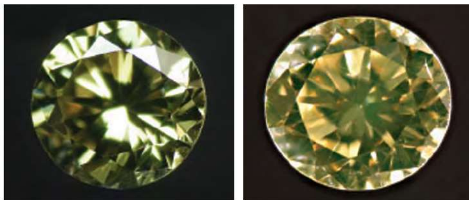
Figure 1. This 0.12 ct diamond, shown on the left in daylight, exhibits green transmission luminescence in dark-field illumination (right), as well as an unusual combination of absorption features. Photos by T. Hainschwang.
