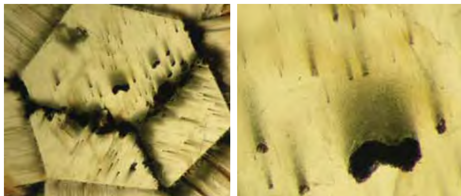
Figure 9. As seen here in transmitted light, two sets of growth channels are apparent in the trapiche tourmaline (left), one following the vertical growth direction of the pyramidal faces, and one nearly perpendicular to the prism. Some channels are empty, while others are filled with a black carbonaceous material (right). Photomicrographs by T. Hainschwang; magnified 10 \times (left) and 40 \times (right).
