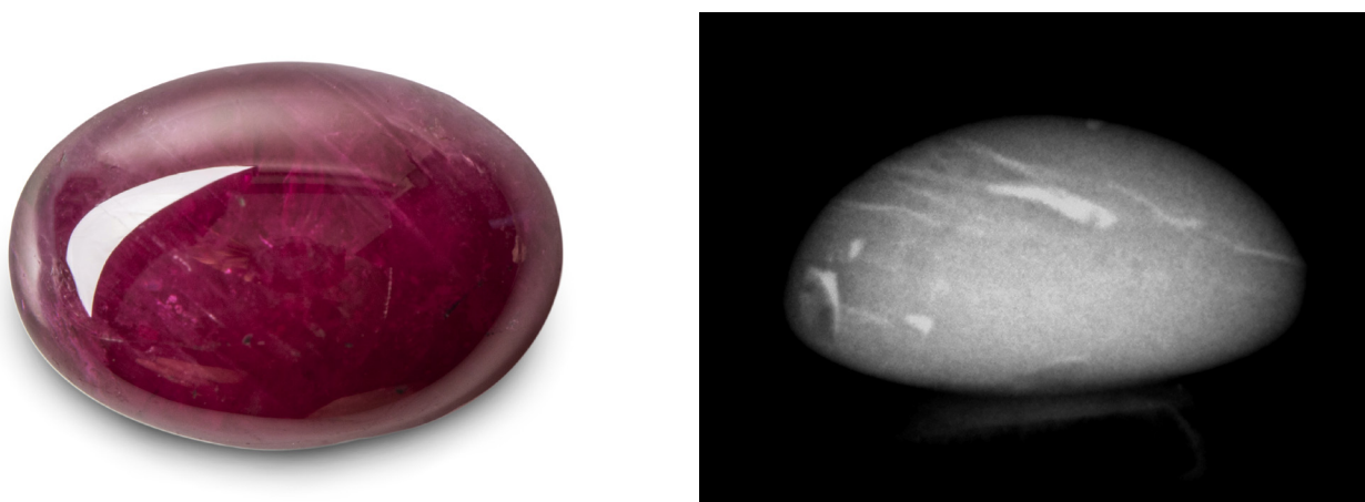
Figure 1. Left: The 3.71 ct barium glass filled ruby. Right: The radiograph showing the filled fissures and cavities of the ruby indicates that the glass contains far heavier elements than the elements usually encountered in corundum (atomic weight from \approx 48 to 70). Photo on the left by C. Nacht, GGTL Laboratories; radiograph by T. Hainschwang.
