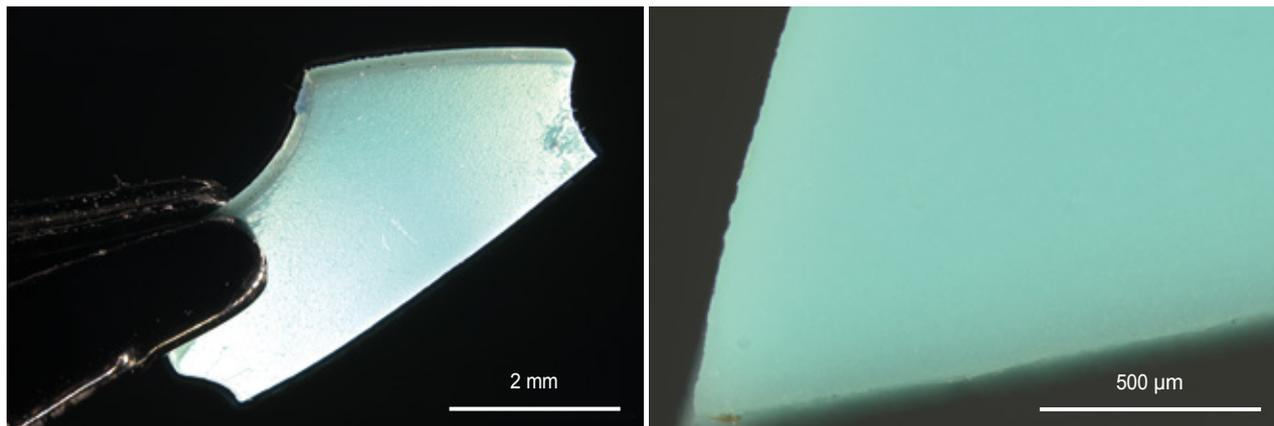
**Figure 39:** Microscopic examination of the turquoise-like specimen shows a glassy lustre (left) and extreme homogeneity, even at the highest available magnification (right). Photomicrographs by F. Blumentritt.
