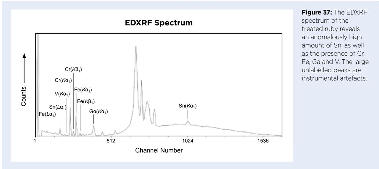
**Figure 37:** The EDXRF spectrum of the treated ruby reveals an anomalously high amount of Sn, as well as the presence of Cr, Fe, Ga and V. The large unlabelled peaks are instrumental artefacts.
