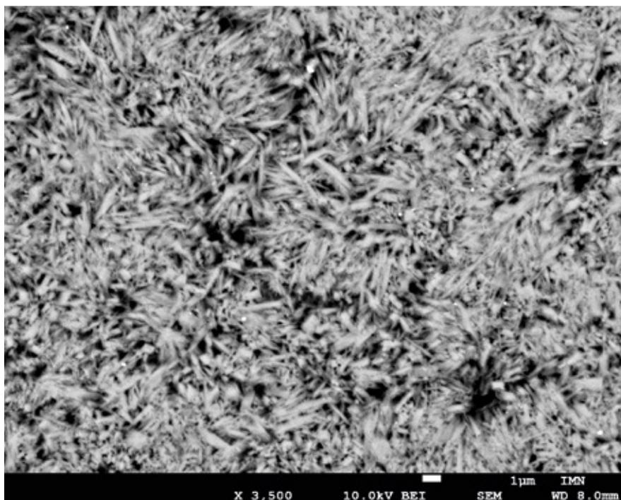
**Figure 41:** In this SEM image of the surface of the sample, use of a backscattered-electron detector, which reflects the chemical composition of the material, shows the global disorder of the turquoise grains (light tones) that are cemented together with organic matter (dark tones). Image by N. Stephant and E. Fritsch.
