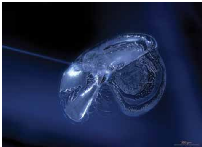
Figure 15 (Three images). Disoid fractures healed during cooling, with formation of synthetic and artificial compounds. (Micrographs courtesy of Patthamaporn Sukkasem)
