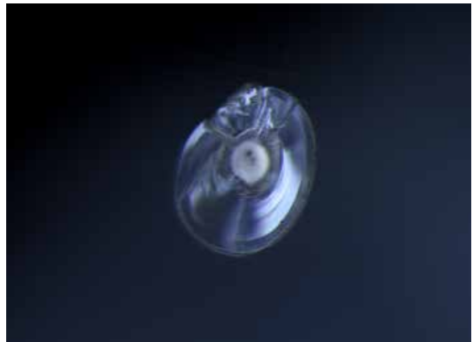
Figure 13 (Three images). "Snowballs" which show the zone of miscibility of chemical rearrangements between the inclusion compounds and those of the corundum.
