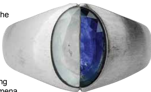
Figure 7. Example of color creation: An oval gray and opaque "Geuda" sapphire was faceted and then cut in two parts. One half was heat treated at high temperature (right); it became blue and transparent. (Photo: Coralie Nacht)
