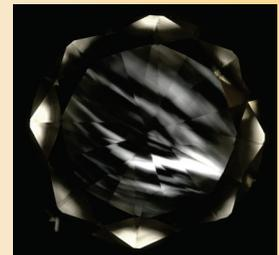
**Figure 1:** The first melee-sized (1.6 mm diameter) colourless CVD synthetic diamond, not treated post growth, as seen under crossed polarizing filters. The gray to black lamellar extinction bands are characteristic for CVD synthetic diamonds.
